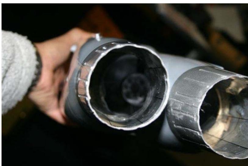
Here's the trunk and fan-unit installed in the fuselage. Hardly any wrinkles. Notice the station-lines on the plastic film.
