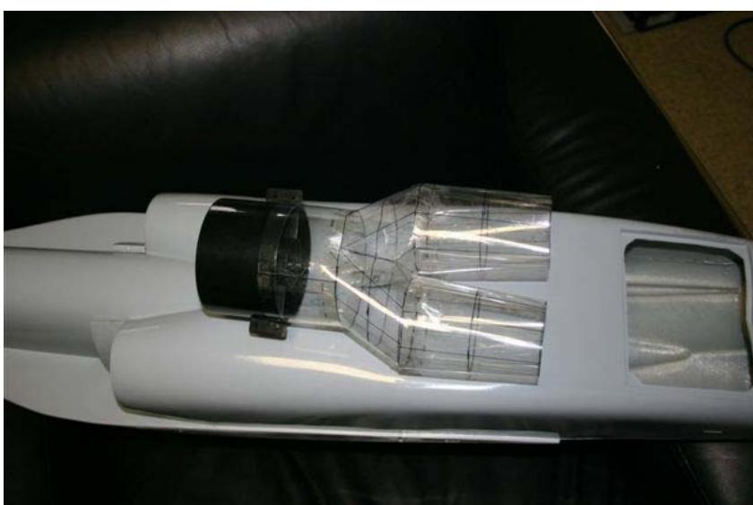
Trunk attached to the fan-unit. Make 10mm slots in the mounting flanges of the fan-unit so that the exhaust can slip over the fan-unit shroud. Install your motor in the fan-unit. Use the installation manual from the fan-unit. Shown here is our 9305 fan-unit.
