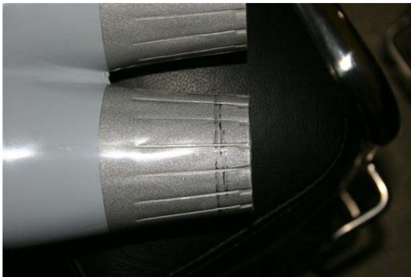
The exhaust must have an inner diameter of approximately 59 mm so you must cut off 18-19 mm from the 2 exhausts.
