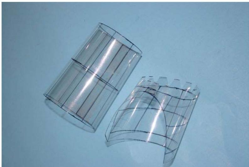
After you have cut out the plastic pieces from the plastic sheet. Tape the pieces together. Like on the left picture. Notice the edge of right piece. Small triangular pieces are cut out.
